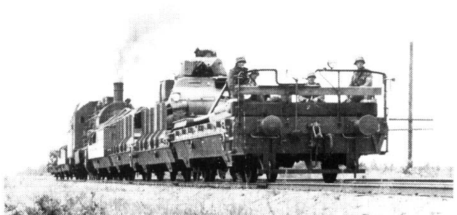
The broad-gauge armored trains PZ 26-31 (here PZ 28) made for the Russian campaign were an unsatisfactory makeshift solution, which consisted of an attack car (in front) and an only partly armored Series 57 locomotive, plus only a tank car (with unloadable captured Somua S 35 tank) and open-top infantry cars (here covered with canvas) with armored sidewalls. (BA)
