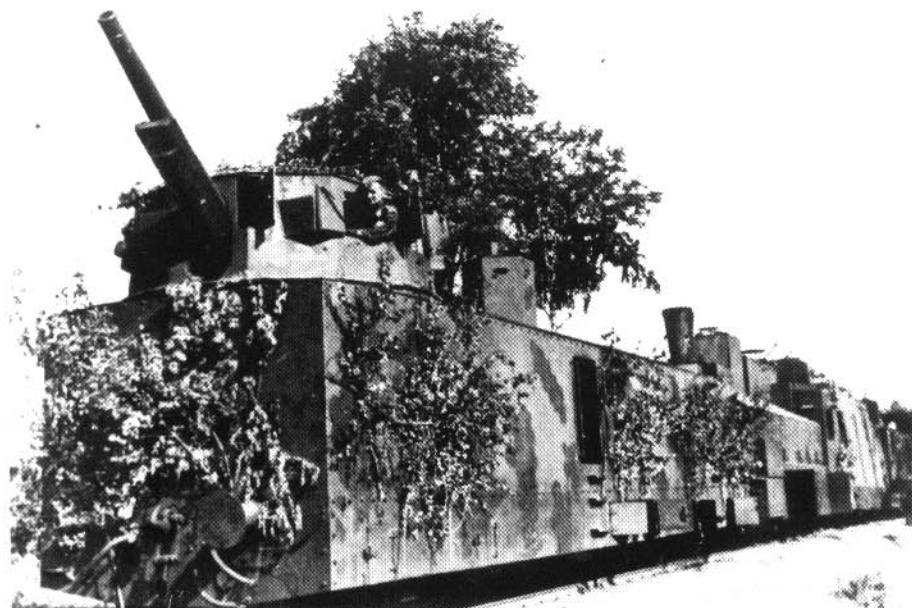
The Armored Train Type BP-35, produced in series on the thirties, is seen above in its light version (Type A) with two turrets per car (7.62 cm 02/ L 39 guns) per car, and below in its heavy form (Type B), with just one turret but a larger-caliber gun (here the 10.7 cm M 10 field gun). (AG & NB)
