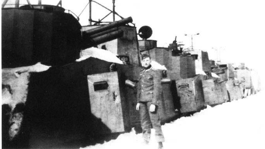
In the immediate prewar era, armored trains were put into service by the NKVD which—though equipped with an additional steam locomotive—had three motorized MBW D-2 motorized cars (two gun turrets each, of the same type as the BP-35). This one was captured in the southern sector of the eastern front in the winter of 1941-42.
